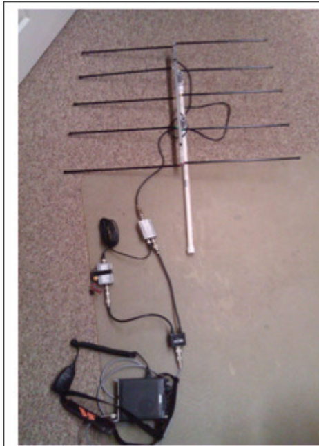
Figure 8: N8MH setup using FT-817, Elk antenna, diplexers, and preamp.
