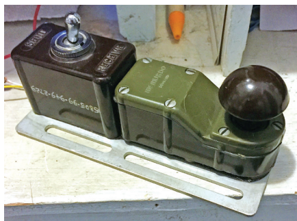
Robert, KI0G, used this World War II British McMurdo key during SKN 2017. [Robert Cutter, KI0G, photo]
