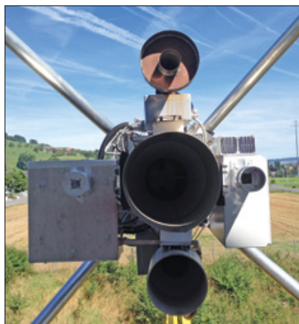
Looking at the business end of the "feed turret" shows how HB9Q puts the big 10 meter diameter dish to work. In the center is the 1296 MHz feed, with the 2.3 GHz feed underneath. On top is the 3.4 GHz feed, at the right is the 5.76 GHz feed, and 10 GHz is on the left. [Daniel Gautschi, HB9CRQ, photo]
