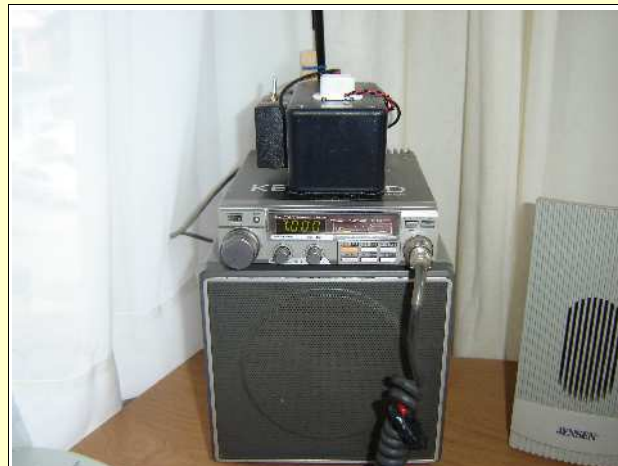
The Kenwood TM201A radio is attached to the Kenwood speaker with hook & loop fasteners. The plastic enclosures are also attached to the radio in this way. This makes a single unit that is easy to service and move for cleaning.
