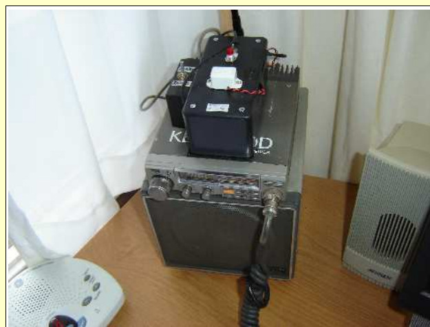
The radio has a whip antenna attached using a right angle connector from the RF UHF connector at the rear. The plastic enclosure has the Sonolert buzzer on top and the red reset button behind it. Further to the rear is a power on-off switch for the alert circuit and an LED to indicate when power is on. The small enclosure on the left houses the "normal/alert" select switch.
