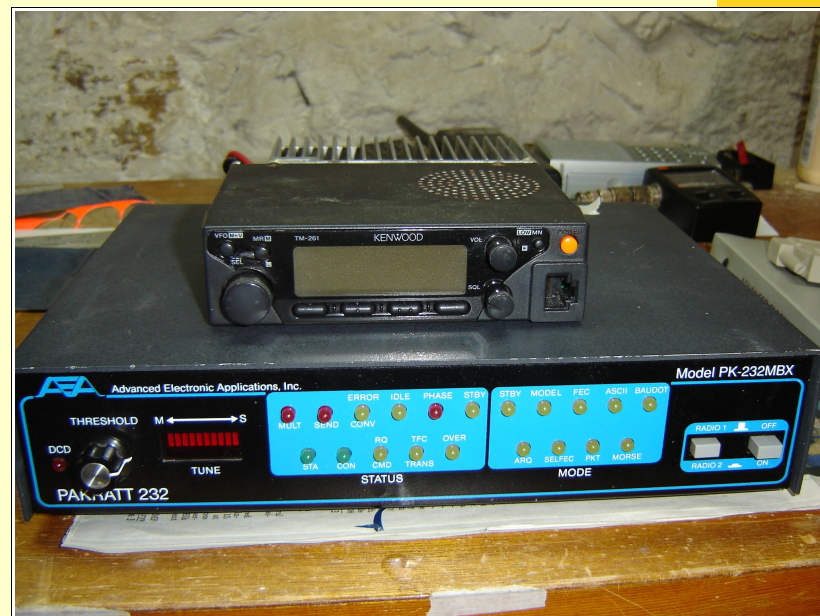
The AEA PK232MBX Terminal Node Controller (TNC) works with a computer and the Kenwood TM-261A 2-meter transceiver. The TNC and radio are both powered from 12 volts. This is the setup used as the WW30 digipeater That relays packet signals around Ridgway, PA.
